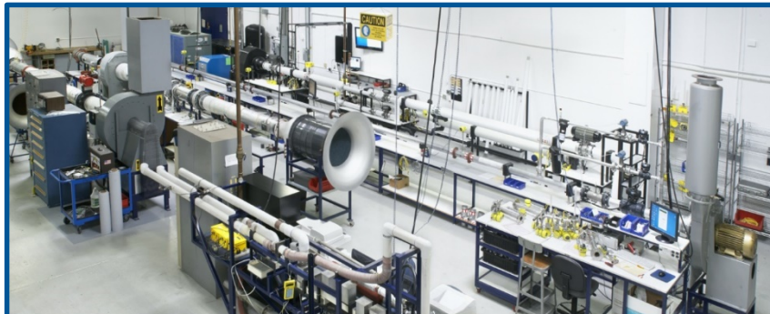
Flat flow profile flow stand (for large diameters)
