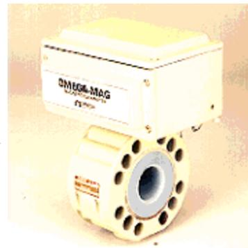
Figure 8: Water-type electromagnetic flowmeter is light weight, compact, and can be easily installed between existing pipe flanges. The no-moving-part instrument has negligible pressure drop and can handle numerous liquids and slurries, provided they are conductive.
