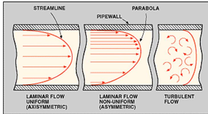
Figure 1: Laminar and turbulent flow are two types normally encountered in liquid flow Measurement operations. Most applications involve turbulent flow, with R values above 3000. Viscous liquids usually exhibit laminar flow, with R values below 2000. The transition zone between the two levels may be either laminar or turbulent.
