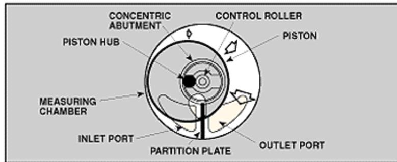
Figure 4: Oscillating-piston meter operates on a magnetic drive principle so that liquid will not come in contact with parts. A partition plate between inlet and outlet ports forces incoming liquid to flow around a cylindrical measuring chamber and through the outlet port. The motion of the oscillating piston in the unit is transferred to a magnetic assembly in the measuring chamber, which is coupled to a follower magnet on the other side of the chamber wall.
