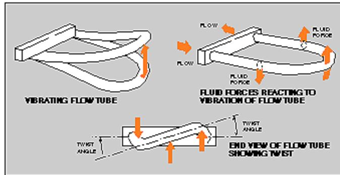
Figure 11: Vibrating, U-shaped flow tube is heart of popular Coriolis mass flow meter. Tube vibration, coupled with the fluid's force, causes tube deflection that is directly proportional to the mass flow rate
