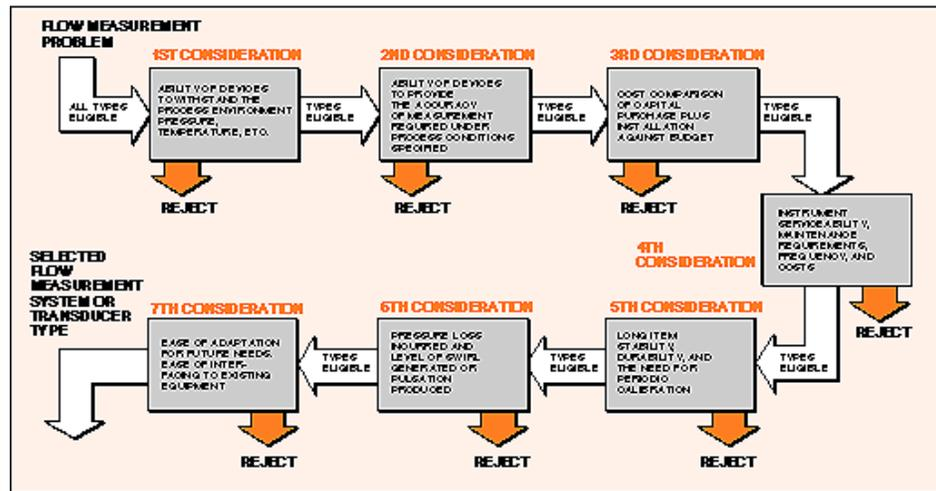
Figure 13: Major considerations involved in selecting flowmeters for a specific applications include serviceability and maintenance requirements.
