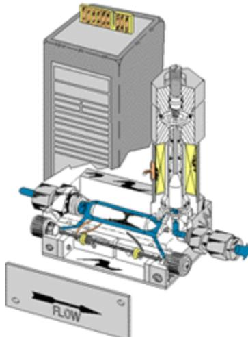
Fig 12: Thermal mass meters utilize a bypass design with RTD sensors to determine the flow rate.
