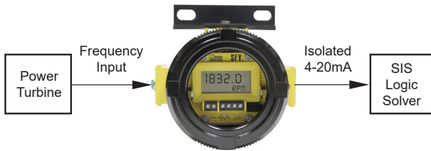
Figure 2. Turbine Over Speed Protection System
