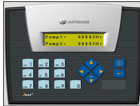
Jazz pump controller indicating individual pump runtimes
