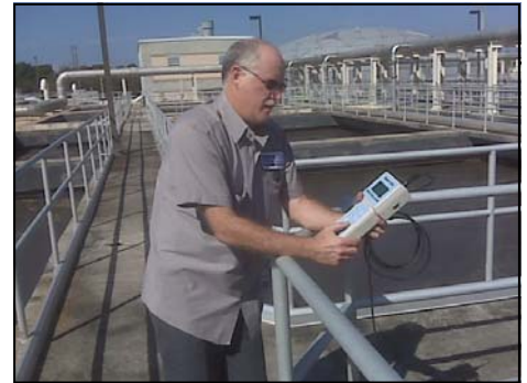
Roger Laferriere of Pinellas County Utilities South Cross Bayou WRF takes DO reading
