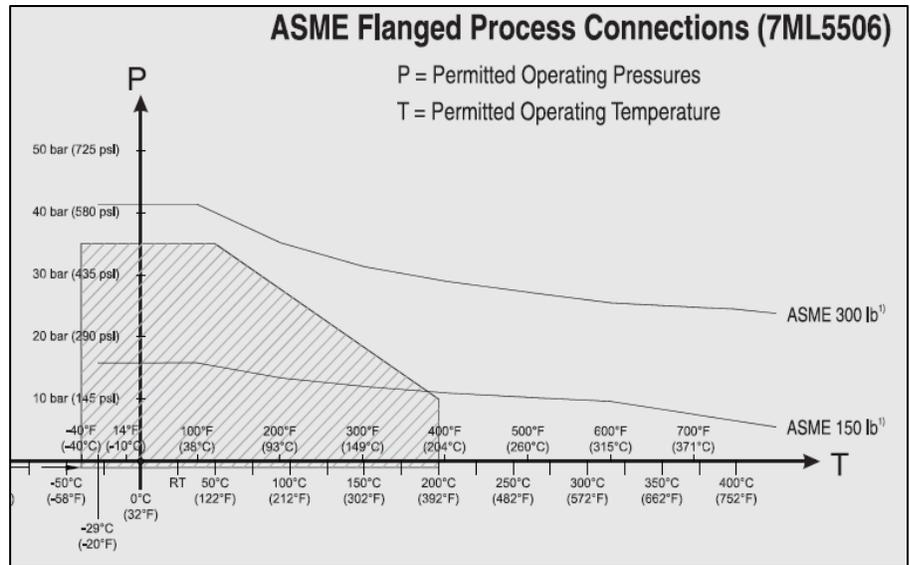
Fig. 2, De-rating table for flange on level transmitter
