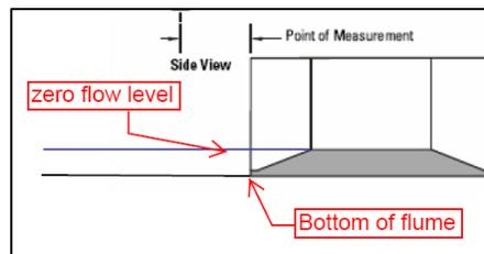
Fig 1. Zero-flow level is not bottom of Palmer Bowlus flume
