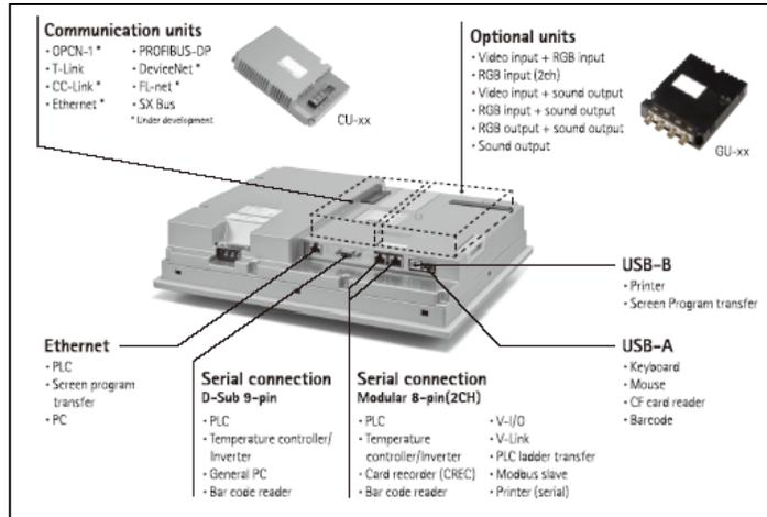
Connectivity to peripheral equipment via the multiple communications ports
