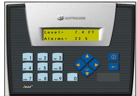
Unitronics controller with pump control software
