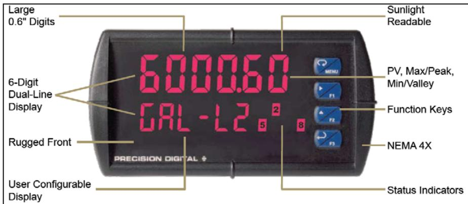
Three function keys on the front panel can be configured to acknowledge alarms, reset max/min, disable/enable output relays, and hold outputs. These events can also be triggered remotely using ProVu's digital I/O module. This capability could provide a remote means for disabling all output relays, for example (interlock, safety).
