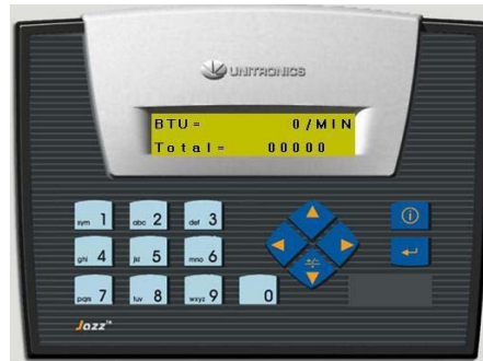
BTU meter displaying rate and total
