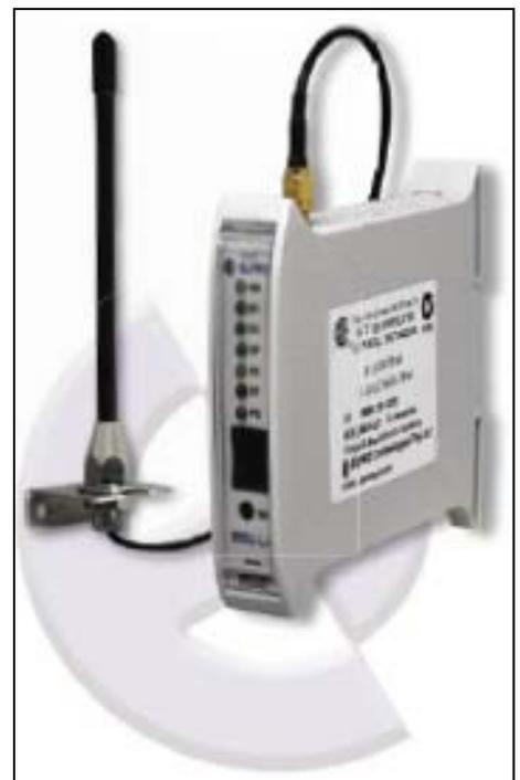
The L-Series transmitter is the first I/O product to allow temperature sensor inputs. Cold junction correction and linearization are performed on the module and may be sent to any of the I/O product output points, or to a Gateway without any additional conditioning. When combining a 4-20mA input simultaneous with a t/c input, many monitoring applications are possible like temperature compensated flows.
