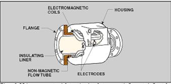
Figure 9: Major components of obstruction-free electromagnetic flowmeter's flow tube include electrodes and coils.
