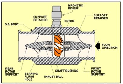
Figure 5: Turbine flowmeter consists of a multiple-blacked, free-spinning, permeable metal rotor housed in a non-magnetic stainless steel body. In operation, the rotating blackes generate a frequency signal proportional to the liquid flow rate, which is sensed by the magnetic pickup and transferred to a read-out indicator
