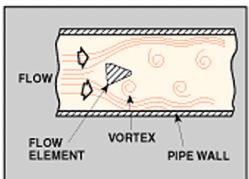
Figure 6: Vortex meters operate on the principle that when a nonstreamlined object is placed in the middle of a flow stream, a series of vortices are shed alternately downstream of the object. The frequency of the vortex shedding is directly proportional to the velocity of the liquid flowing in the pipeline
