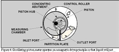
come in contact with parts. A partition plate bet ween inlet and outlet ports forces incoming liquid to flow around acylindrical measuring chamber and through the outlet port. The motion of the oscillating piston in the unit is transferred to a magnetic assembly in the measuring chamber, which is coupled to a follower magnet on the other side of the chamber wall
